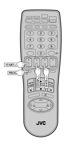
You can directly program the VCR's timer to record up to 8 shows, as far as a year in advance. Remember, the clock must be set before you can program the timer ( pp. 6 or 9).
