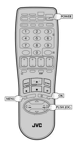
The Plug & Play function simplifies installation by guiding you through the procedures of setting the language, clock and tuner channels — simply follow the on-screen menus that appear when the **POWER** button is first pressed to power on the VCR after you connect the power plug to an AC outlet.
