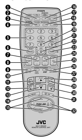
Buttons with a small dot on the left side of the name can also be used to operate your TV after having pressed the **TV** button. © pg. 41
